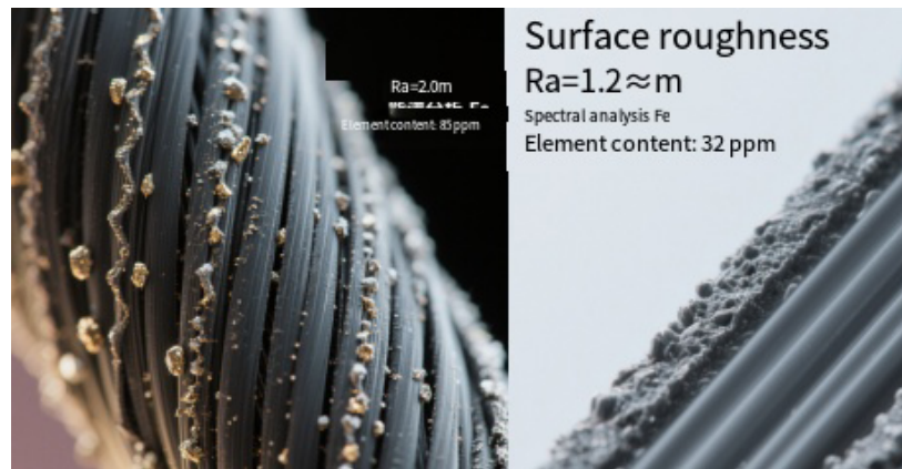
Figure 2. SEM images of the surface of carbon fibers prepared from filaments with different impurity contents.
